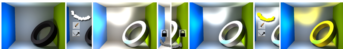
Figure 2.3: Creation of a caustic from two input strokes [Ngu13]. The chosen interaction mode is indirect, which instructs the algorithm to optimize lighting away from the pointer location.
