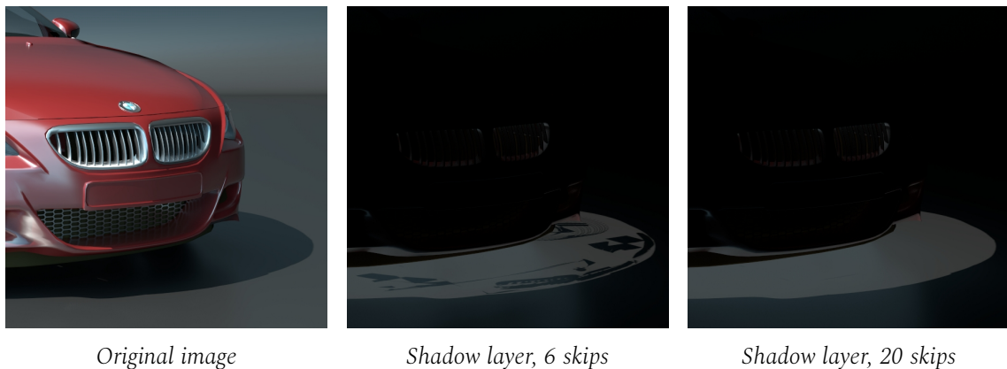
Figure 4.14: If the maximum number of skips is too low, the shadow layer displays characteristic bias where paths are terminated before reaching a light source.
